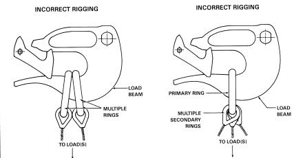
Figure 2-1. External load rigging
