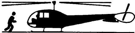
3. Approach or leave in pilot's field of vision (to avoid tail rotor).
