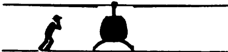
5. Hold onto hard hat when approaching or leaving machine, unless chin straps are used.
