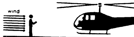
13. When directing machine for landing, stand with back to wind with arms outstretched toward landing pad.
