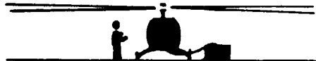
12. After hooking up cargo sling, move forward and to side to signal pilot (to avoid entanglement and getting struck, with loaded sling).
