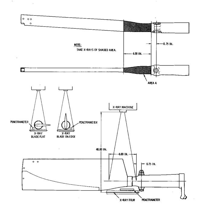
Figure 1. Tail Rotor Blade and Spar X-ray Setup and Area (Sheet 1 of 3)
