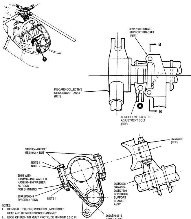
Figure 1. Installation of Collective Stick Support Bracket Reinforcement Strap
