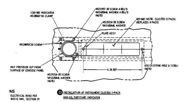
Figure 1. Instrument Cluster 4-Pack Conversion (sheet 3 of 3)
