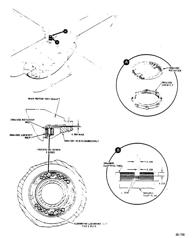
Figure 1. M30223 Kit Installation - Main Rotor Hub Locknut and Retainer Ring.
