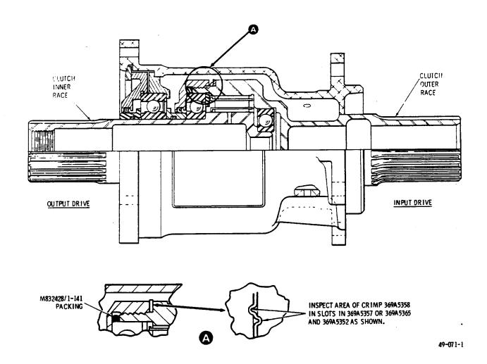
Figure 1. Inspection of Overrunning Clutch Assembly and Engine Output Drive Splines.
