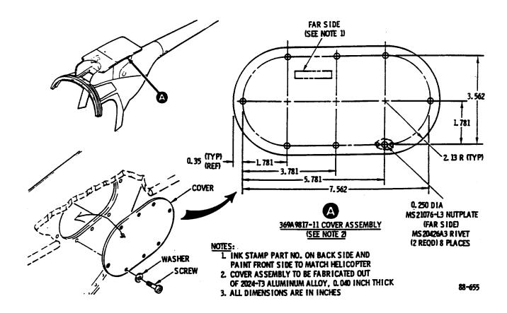
Figure 1. Fabrication of 369A9817-11 Cover Assembly.
