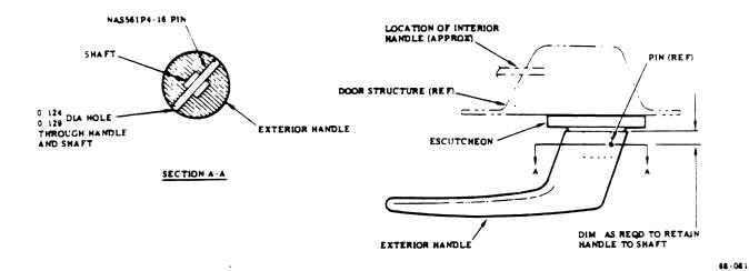
Figure 1. Modification -Door Latching System (Autolatching), Pilot and Cargo Doors
